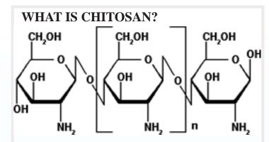
Chitosan (shown above) is a natural biopolymer derived from chitin - the structural material found in crustaceans. Found naturally in the environmental, chitosan is 100 % biodegradable. Chitosan is a long chain polymer and possesses a strong positive charge. Dirt particles typically are negatively charged. Chitosan flocculates (clump together into a large mass) fine dirt particles causing them to settle thereby clarifying the dirty water. (See before and after treatment below.)
