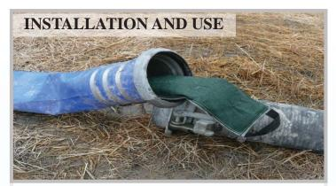
Simply anchor the cartridge in flowing dirty water and it will convert into a slow-dissoloving gel. As it dissolves, chitosan is released into the water causing fine sediment particles to flocculate. Once treated, water can be gravity settled, biofiltered, infiltrated, sand filtered or filtered by a dewatering bag. Visit our website for more information to assist with installation and maintenance.
